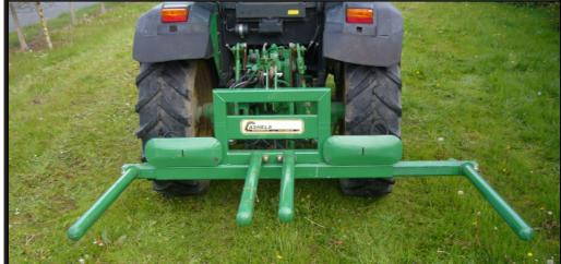
The Cashels Hydraulic Vari-Width Double Bale Handler has been developed to cater for the transport of two 4 foot wrapped bales without damage to film. This new innovative design enables the farmer/contractor to minimise the time from field to storage, without compromise to bale integrity.
